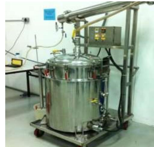
For this technology, a supercritical-fluid extractor is required and it consists of a tank of the mobile phase, usually CO<sub>2</sub>, a pump to pressurize the gas, an oven containing the extraction vessel, a restrictor to main high pressure in the extraction line, and a trapping vessel. Analytes or extracted components are collected by letting the solute-containing supercritical fluid decompress into an empty container, through a solvent.
