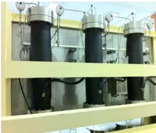
A research hub was established between IMU and SRAS Berhad in 2013 and under this partnership, SRAS has made available its Supercritical Fluid Extraction System (SCFS) in its GMP facility. The SCFS allows the rapid, efficient, economically competitive and environmentally friendly method to extract reasonably large amounts of analytes or components from complex mixtures such as herbal compounds, food products, wastes, etc. This has enormous applications to research and industry.
